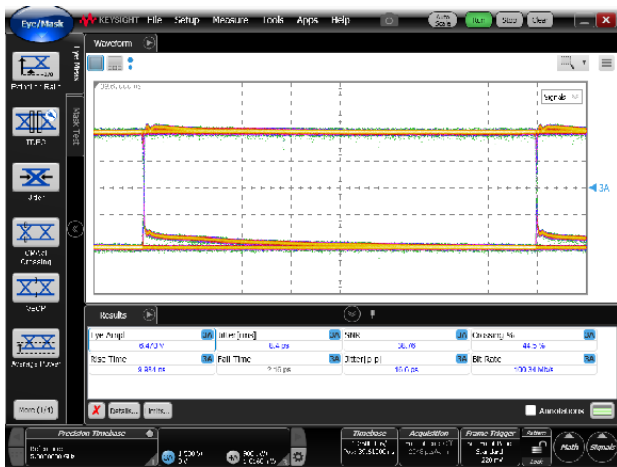
Data Rate = 100 Mb/s, V_{in} = 220 \text{ mV}_{pp}
